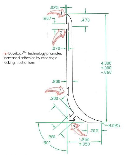
(3) Cove Anchor serves to both anchor the base of the cove to the floor and wall interface, and to lock-out moisture intrusion.
